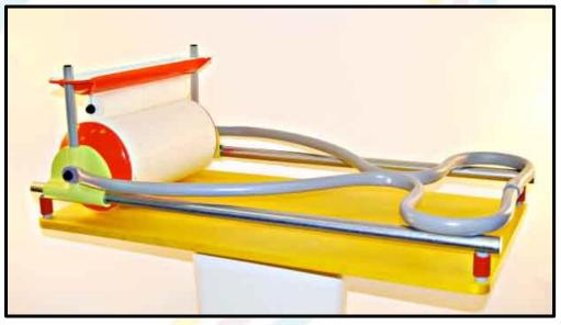
The Tabletop Printer is a portable, fully accessible print table. Participants create their own print plate, which is attached to the print drum, "inked up" with acrylic paint, and their unique design is printed on paper or fabric.
